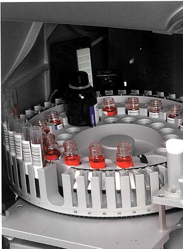
Carousel with random positioning of samples and reagents
